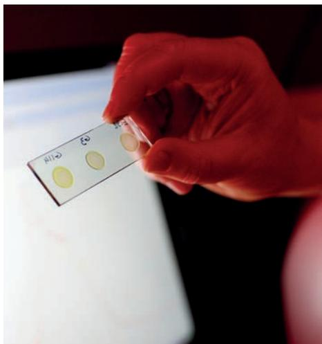
*Pictured above: Spots of blood serum on a slide prior to analysis using Raman spectroscopy, which generates a biomolecular fingerprint of the specimen. This spectral fingerprint can then be analysed to extract screening/diagnostic features of Alzheimer's disease.*
